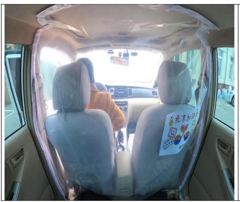
A cab driver has used a thick plastic sheet here to separate himself from the passenger. AC would remain switched off (even in those cars that have separate read vents). Only one driver and passenger could be allowed. If four separate enclosures are made – four passengers could be allowed with staggered entry only. That would need RTA office approval though.
